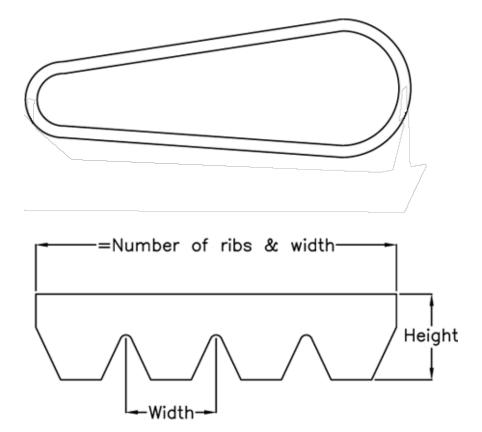
$\begin{array}{ll} \text{Datum Llength} = 4470 \\ \text{Height} &= 16.5 \\ \text{Number of ribs} = 8 \\ \text{Pitch} &= 9.4 \end{array}$
